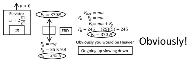
Find the weight of a 25 kg object on a scale in an Elevator moving down,  $a = 2 \frac{m}{s^2}$  downward.
