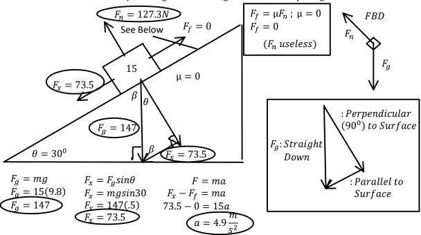
What is the acceleration of a 15 kg block sliding down a  $30^{0}$  slope with  $\mu = 0.3$ .
