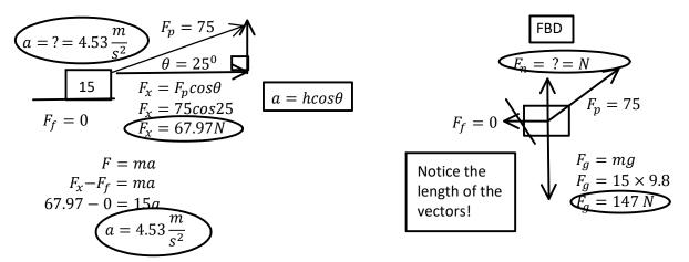
Find the "a" of a F = 75 N on a 15kg object pulled at an angke of 25° and  $\mu = 0.2$ ? in diagram.
