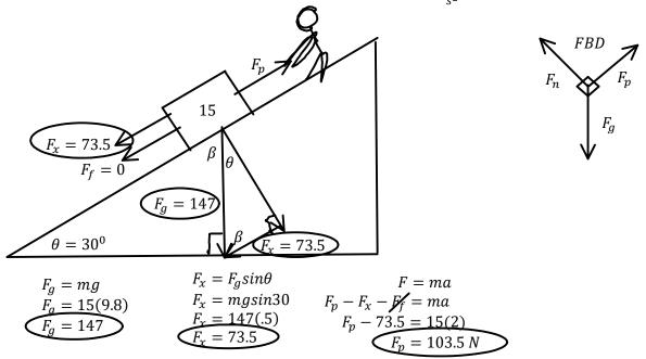
How much force is required to accelerate a 15 kg object at  $2\frac{m}{s^2}$  up a slope  $30^0$  with  $\mu=0.3$ ?
